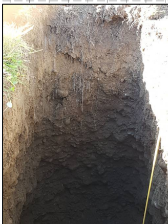
Excavator met target depth. at 2 m. Scala Penetrometer met practical refusal at 0.6 m depth. Standing groundwater was not encountered
