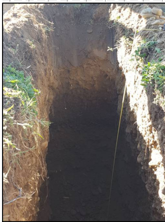
Excavator met target depth. at 2 m. Scala Penetrometer met practical refusal at 0.7 m depth. Standing groundwater was not encountered
