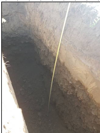
Excavator met target depth. at 2.2 m. Scala Penetrometer met practical refusal at 0.9 m depth. Standing groundwater was not encountered
