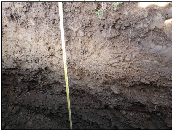
Excavator met target depth. at 2.1 m. Scala Penetrometer met practical refusal at 0.4 m depth. Standing groundwater was not encountered
